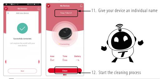
If you have any problems connecting to the robot, check your Wi-Fi connection and password. Uninstall and reinstall the app if necessary. Press the Power and HOME buttons at the same time.
